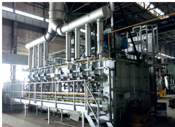
Double chamber forging furnaces; 2 doors
