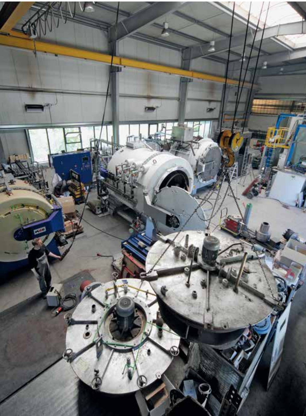
Final assembly of the nitriding furnaces and special systems
