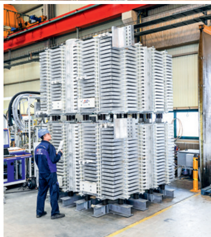
Walk-through aluminium casings for a Spark gap - for controlled discharges for Series capacitors in power distribution boxes
