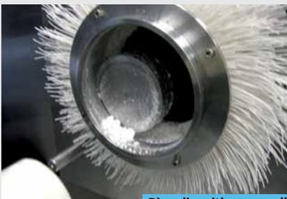
Ring die with press roller and supply tube
