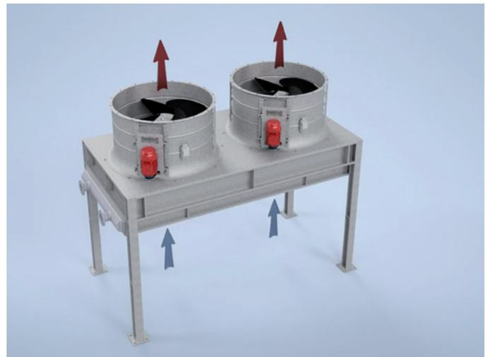
The induced arrangement of fans, positioned above the heat exchanger bundles, ensures a very uniform flow over the heat transfer surface. The shading of the heat exchange bundles provides protection against intense sun radiation.
