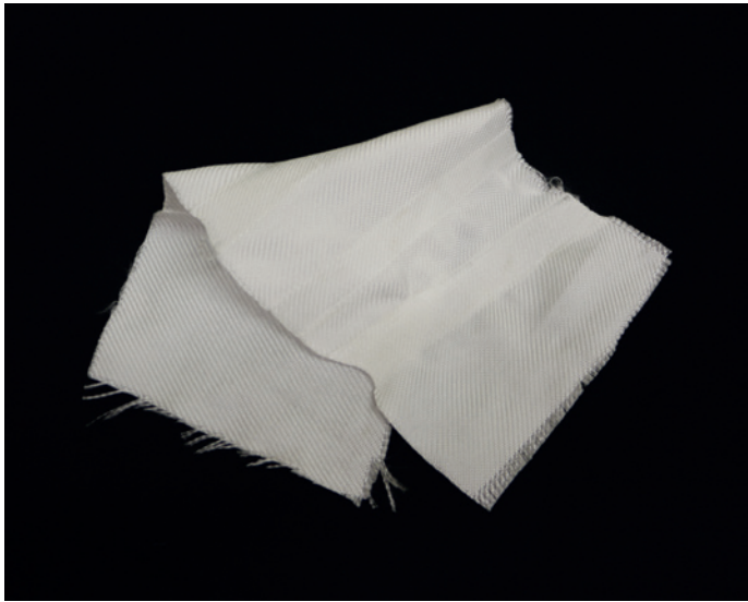
Fig. 2: srPLA fabric with directly integrated stiffening ribs through partial consolidation
