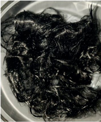
Fig. 1: Reclaimed 2 nd life carbon fibre after solvolysis treatment
