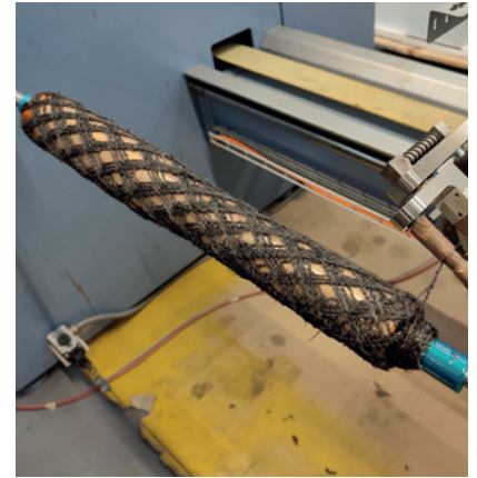
Fig. 3: Manufacturing of tubular sections via dry filament windin
