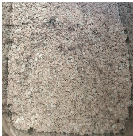
Fig. 2: Compounding tests left: NF/PP-PE flakes with low bulk density; right: Compounder with feed screw (red) for material dosing
