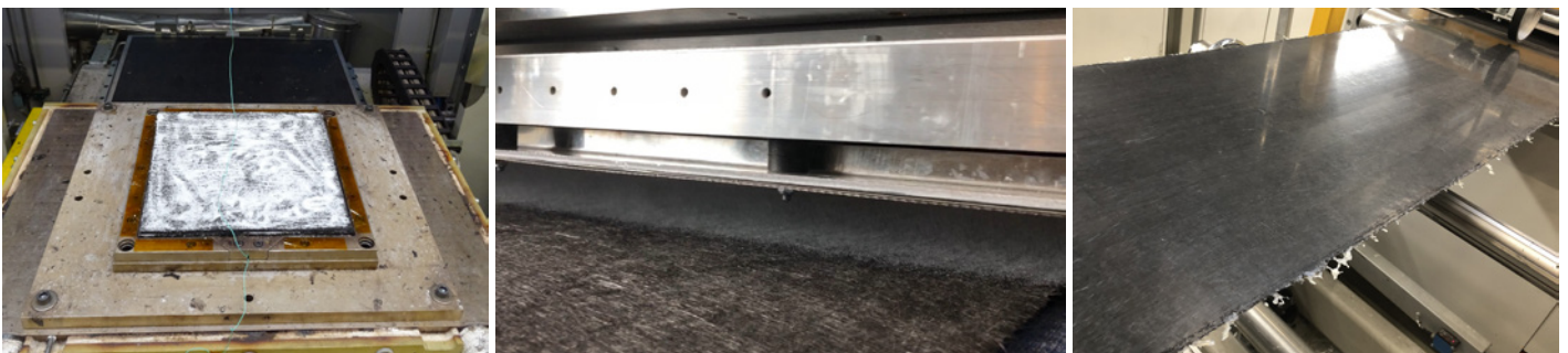
Fig. 2: Manual powder impregnation at IGCV for test panels, showing the scattered powder before heat pressing (left), Automated powder impregnation (middle), Organosheet production (right) [1]
