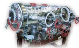
Heating jackets and heating tapes to bake out vacuum components. for temperatures up to 450 ° C.
