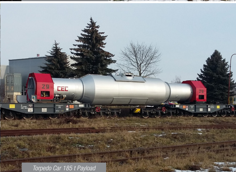
Torpedo Car 185 t Payload
