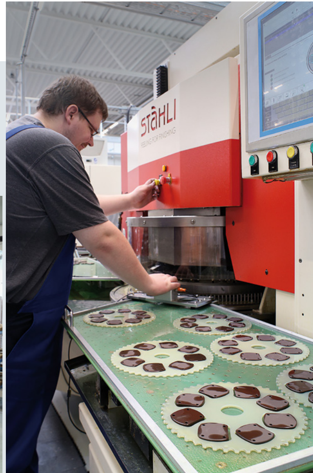
The sintered parts are then ground and polished.
