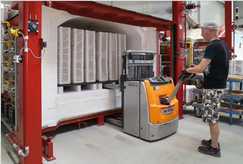
The pressed parts are fired in the oven.
