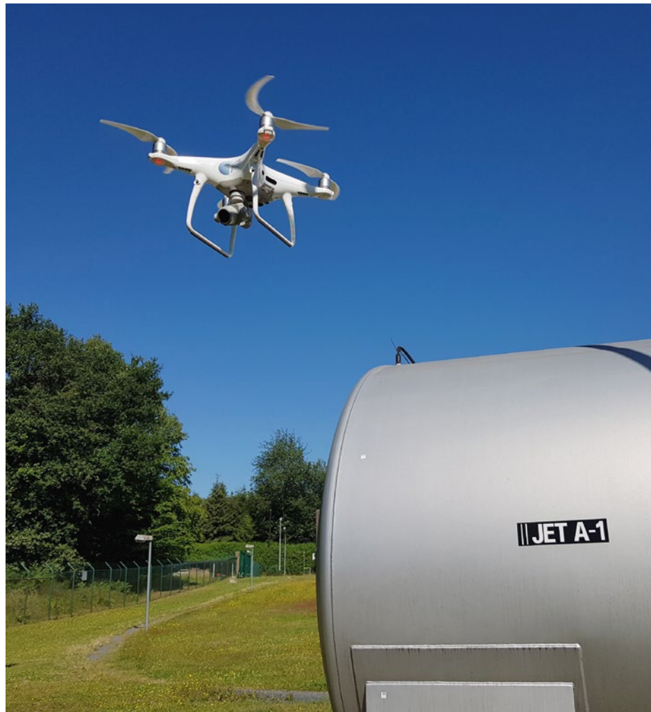
Pipeline protection and inspection by Unmanned Aerial Vehicle
