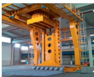
Chargemaschine Tragkraft: 20t
