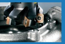
Accurate finest metered lubrication dramatically reduces friction in the working areas. The absolutely unique nozzle technology allows the lubricant to penetrate the high centrifugal forces acting during high-speed machining. The result: The lubricating effect can develop to the full.
