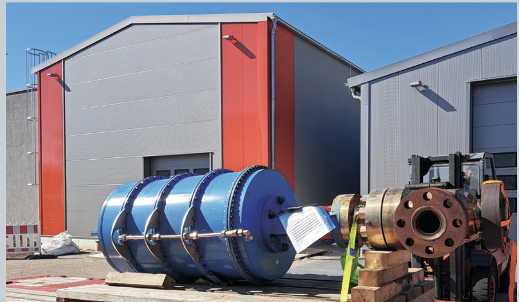
High-pressure angle valve in service for over 20 years shipped to VETEC as part of routine revision activities
