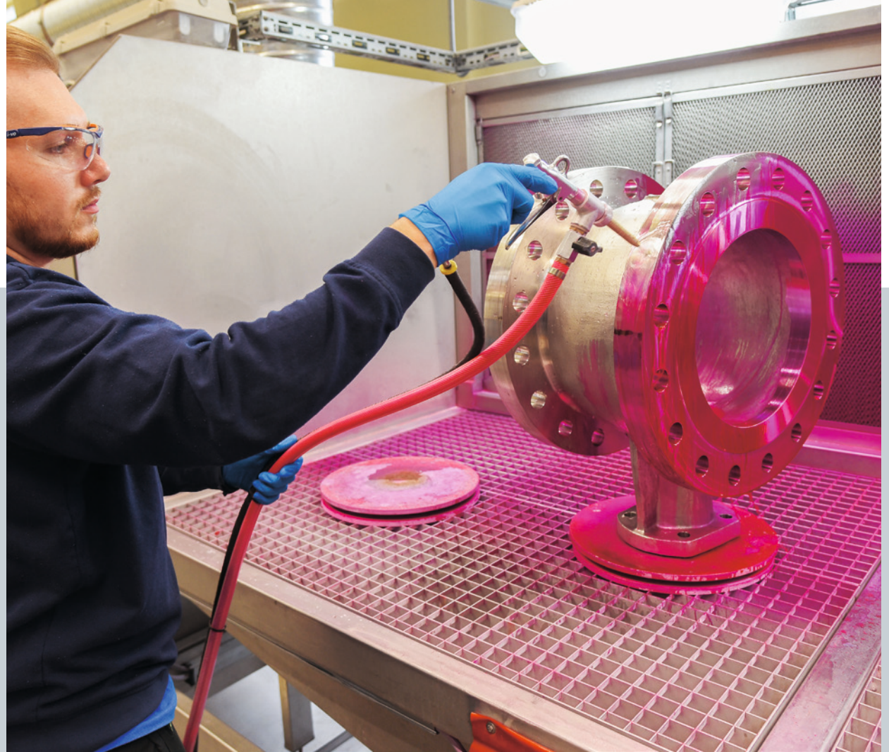
Dye penetrant test performed on a valve body
